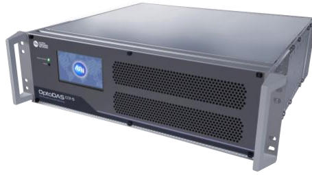
Figure 4: An example of a DAS interrogator unit. Similar interrogator units are used for Brillouin and Raman OTDR. Source: ASN.
